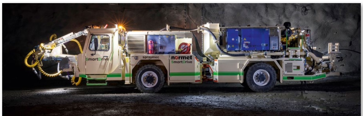
Fig. 4: The traction batteries used in the heavy-duty commercial vehicles from the M-range from Normet are 90 kWh batteries with 23Ah High Energy LTO cells from Toshiba.
